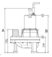
unit : mm C.W.L : Continuous running water level L.W.L : Lowest running water level
